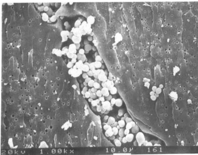
FIGURE 8 SEM micrographs of chloroform-extracted 10 wt.% Udel® blended samples after immersing for 10 minutes.
